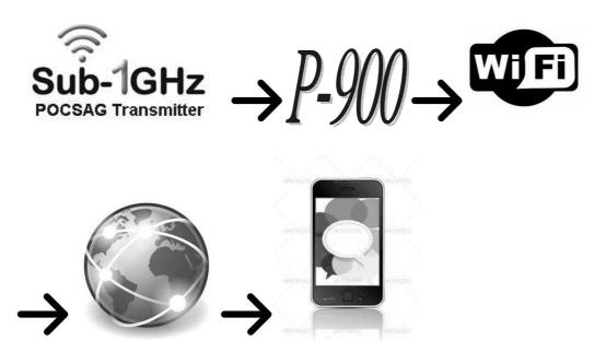
a. Sub-1GHz POCSAG transmitter (148,315,433,426,457,868,915...MHz)
