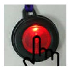
8-3. Test the peripheral and just add to activate the peripheral again. If added successfully, the mobile device should be getting a message.
