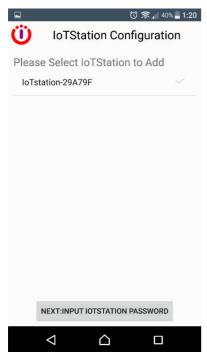
6-5. Step5: Select the IoTStation to add, and click on "NEXT:INPUT IOTSTATION PASSWORD"
