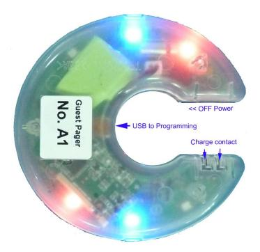
Photo 2 shows the Charging Method and Donuts Pager in / out.
